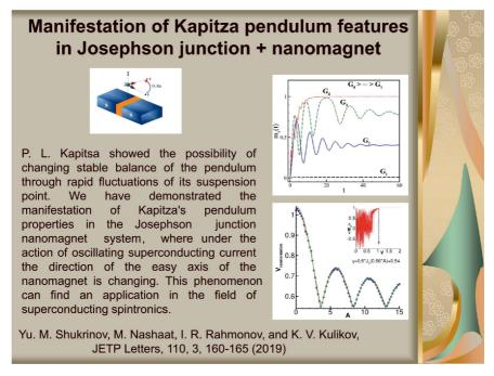
Fig. 16. Dynamics of the magnetization  $m_z$  of the nanomagnet as a function of Josephson to the magnetic energies ratio G, demonstrating its reorientation. The second figure shows the reorientation voltage as a function of the amplitude (A) of the external AC drive. The inset demonstrates the averaged component of the magnetization  $m_z$  of the nanomagnet as a function of the DC voltage
