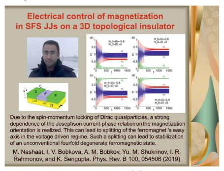
Fig. 14. Sketch of the system considered in Ref. [18]. Superconducting leads and a ferromagnetic inter-layer are deposited on top of the topological insulator. Figure shows the time evolution of the magnetization starting from different initial conditions, corresponding to four possible stable states
