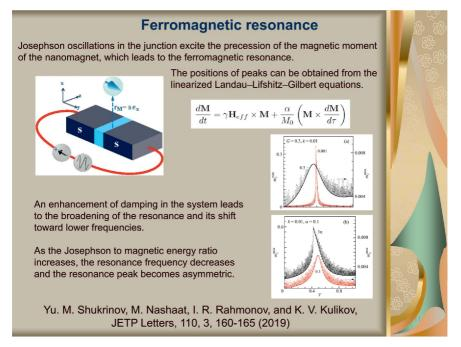
Fig. 15. Manifestation of the ferromagnetic resonance in the dependence  $m_z^{\rm max}(V)$  at different values of Gilbert damping  $\alpha=0.001,0.3$  and two different ratios of Josephson energy to the energy of the nanomagnet  $(G=0.1 \text{ and } 3\pi)$
