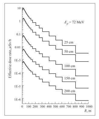
Fig. 1. The spatial distributions of the skyshine-neutron effective dose rate against the thickness of the upper concrete shielding of the DC-72 cyclotron
