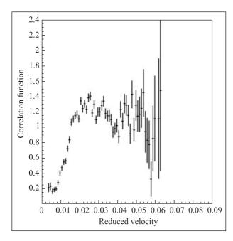
Fig. 8. The correlation function of fragments depending on the relative velocity. Its value is proportional to the probability of the fragment pair production with the given relative velocity
