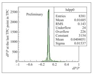
Fig. 6. The relative momentum resolution for charged particles
