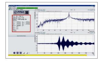
Fig. 10. A tune measurement using «Chirp» excitation (courtesy of the CERN AB/BI Group). The bottom trace shows the vertical beam response and the top trace is the spectrum of the signal with the vertical tune peak
