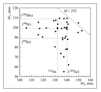
Fig. 3. Results obtained at the COMETA setup: mass-mass distribution of the FFs from  $^{252}$ Cf (sf) when three neutrons (n = 3) were detected in coincidence and an additional selection with the gate in the ( $V_1$ - $E_1$ ) distribution
