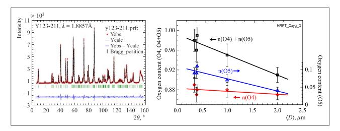
Fig. 1. Left: diffraction spectrum of YBa<sub>2</sub>Cu<sub>3</sub>O<sub>y</sub> sample (annealed at 930 °C with an average crystallite size  $\langle D \rangle = 2~\mu m$ ) obtained on HRPT (PSI, Switzerland) and treated by the Rietveld method. Right: site occupation factors for O(4) (left scale), O(5) (right scale) and their sum (left scale) as a function of the average crystallite size. Statistical errors of the points are indicated. Lines are drawn by the least squares method
