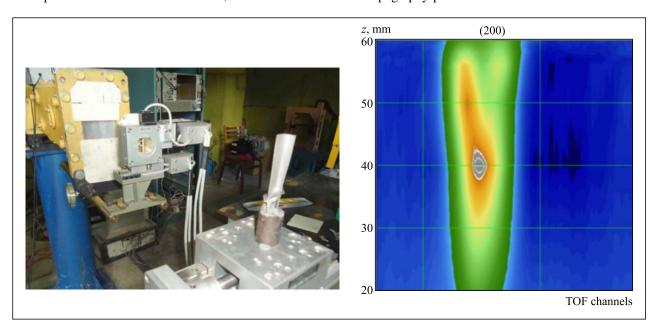
Fig. 2. Left: a turbine blade fixed on the goniometer of the FSD diffractometer for the experiment on the analysis of its microstructure. Right: 2D cross section of the region of the diffraction peak (200) revealing its complex topology. In particular, the presence of a grain with different (compared to the basic matrix) orientation can be seen
