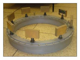
Fig. 4. The ring-shaped detector with 12-channel signal-shaping amplifiers mounted on its case
