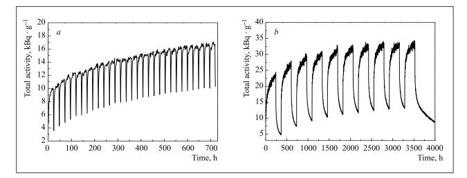
Fig. 14. The dynamics of induced activity accumulation in a beam catcher: a month-long operation at 22 hours of work and a two-hour break per 24 hours (a); 10-year operation at eight straight months of work and a four-month break a year (b)
